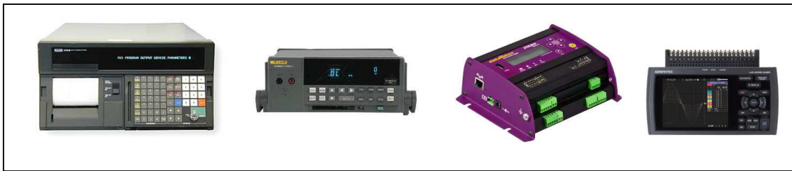
Figure 2. Examples of centralised logging systems
